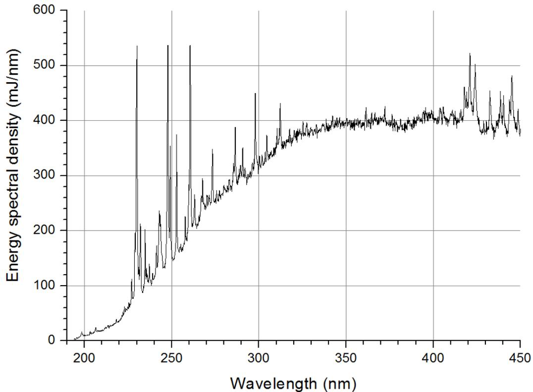
Figure 1. Irradiation spectrum of pulsed xenon unit "Yanex-2"
