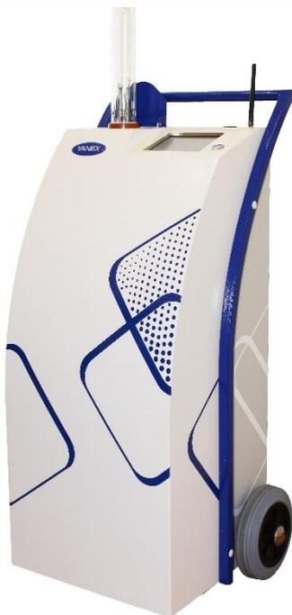
*Pic: The Yanex Pulsed-Xenon UV robots deployed in Netcare hospitals use high doses of UV light to destroy viruses, bacteria and fungal spores and disinfect hospital wards, theatres and other spaces within minutes.*
